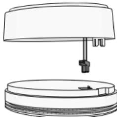
Remove the back cover from the Ei Electronics detector. The GSM communicator will be used as back cover.
