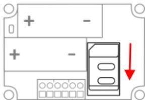
NB: Make sure the SIM card is inserted before the batteries are inserted. In case of a SIM card change, please first remove the batteries (and remove any other external power supply).
