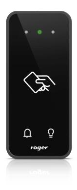
The MCT80M-BLE is an access terminal dedicated to RACS 5 access control and building automation system. Terminal enables identification of users by 13.56 MHz MIFARE® Ultralight/Classic/DESFire/PLUS cards and by use of smartphone with NFC or Bluetooth technology. In case of Bluetooth identification the reading range can reach up to 10 meters while other methods offer few centimetres of reading range. The mobile identification requires Roger Mobile Key application installed on
