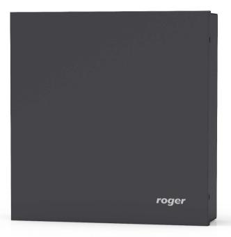
Access control kit designed to support two doors in the ST version of RACS 5 v2 system. The kit includes a metal enclosure with a power supply, a networked access controller, and an I/O expander. The set supports two read-in/read-out doors using RS485 readers (MCT series readers or OSR readers equipped with OSDP protocol), RACS CLK / DTA (PRT series readers), or readers
