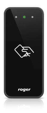
The MCT80M is an access terminal dedicated to RACS 5 access control and building automation system. Terminal enables identification of users by means of 13.56 MHz MIFARE Ultralight® and MIFARE® Classic cards. MCT80M is equipped with RS485 interface which is used for communication with access controller. Be-
