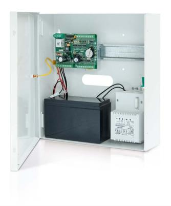
PR402DR-SET consist of PR402DR-BRD access controller module and TRP 40/16/18 power transformer factory preinstalled in ME-1 metal enclosure with space for 7 Ah/12 V back-up battery and tamper contact.
