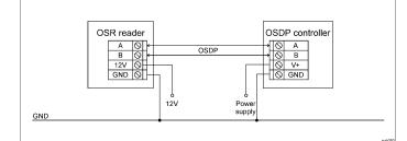
Fig. 3 Typical connection of reader to controller
