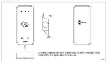
Fig. 2 Enclosure opening and location of service contact
