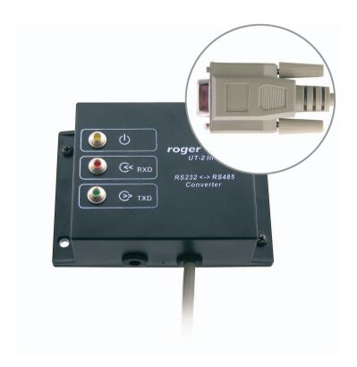
The UT-2 operates as an electrical converter between RS232 and RS485 communication interfaces. It can be used for programming of single access controller or the whole network (subsystem) of access controllers connected RS485 bus. UT-2 device enables bidirectional data transmission between access control devices and management software installed at PC.
