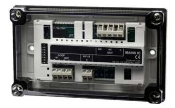
The Mains IO Modules are fully monitored loop powered devices which permit the interfacing of third party equipment with the Fire Alarm Control panel using normally open dry contact connections.
