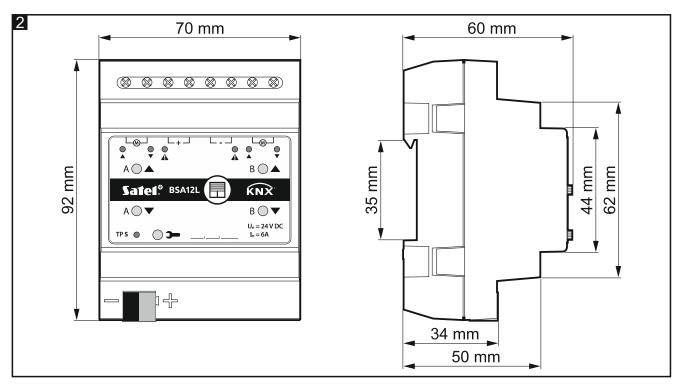
Electronics of the KNX-BSA12L and KNX-BSA12H modules is installed in enclosures of identical shape and dimensions. The enclosures only differ in their panels for manual control of channel state. The figure shows enclosure dimensions based on the KNX-BSA12L module. The module takes up 4 units on the DIN rail (35 mm).
