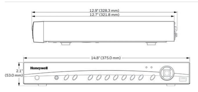
$\textbf{Note:} \ \text{The dimensions of HEN081*3/HEN161*3} \ \text{are shown here.} \ \text{For the dimensions of HEN041*3}, see technical specifications on the next page.}$
