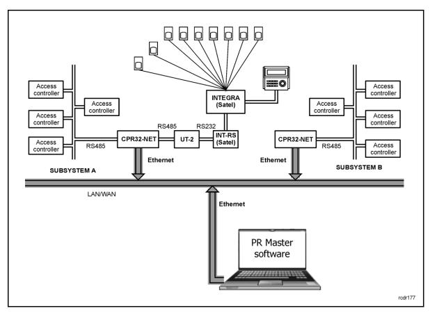
Fig. 1 General diagram of RACS 4 and INTEGRA alarm control panel integration
