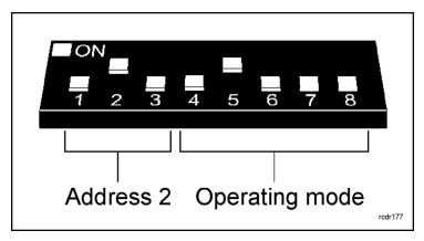
Fig. 3 INT-RS dip switch setting with exemplary address
