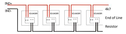
Note: If non-polarised alarm devices (e.g. some types of old mechanical bell, or a relay) are used, then a diode will have to be placed in line with the device to enable fault monitoring. They may also need a back EMF protection diode. (symptoms: Chattering sounder relays that don't turn off).
