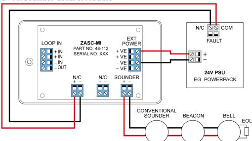
The ZASC requires an external 24vdc power supply (as shown in the above diagram). The EOL for the sounder circuit is  $4K7 \Omega$ . When using the ZASC make sure the PSU being used has a fault output relay, so that in the event of a power supply fault it is reported to the control panel.
