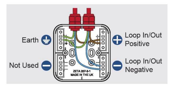
Connecting the sounder is done using the terminals in the back box of the device. Please refer to the above diagram.
