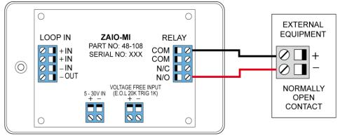
The end of line resistor value is  $20K\Omega$  and the trigger resistor value is  $1K\Omega$ .
