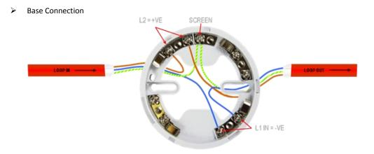
The connection for the detectors bases is made as follows: Terminal L1IN is -ve (Blue) Terminal L2 is +ve (Brown) These are the only two connections required.
