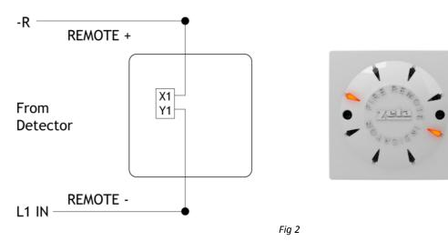
Fig 2: shows the connections for a wall mount version remote LED
