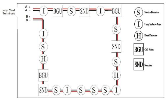
Figure 5: Example of addressable loop wiring (top) & connections to loop cards (bottom)
