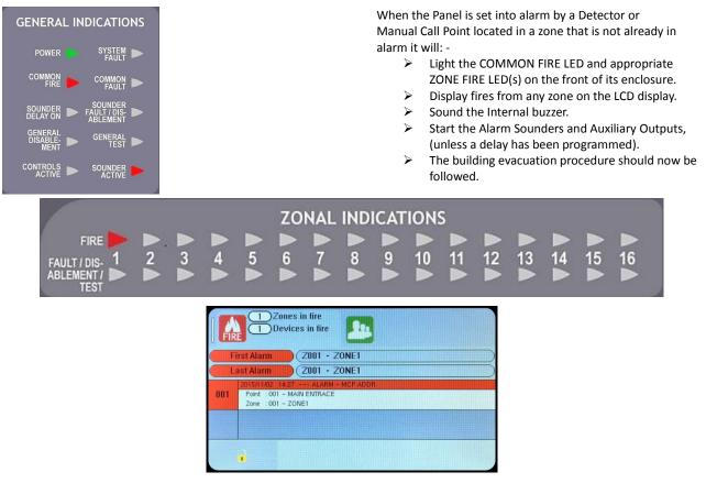
The LCD gives all the alarm information, such as the time & date of the alarm, the address, the device type, the device label, and the zone it is allocated to.
