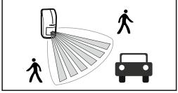
If traffic nearby or objects moving out of the protected area cause an alarm, move the detector slightly downwards or reduce the detector sensitivity.
