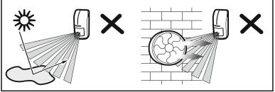
Don't direct the detector on reflective surfaces or on fans or a heat sources.
