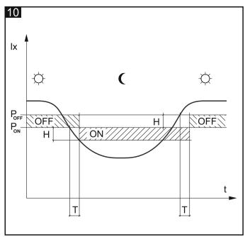
Figure 10 shows the way the dusk sensor operates. On the timeline the T time delay is presented (in operating mode T=15 min, in configuring mode T=3 s). Illustrated with the letter H in Figure 10 light intensity hysteresis and time delay make the sensor immune to short and accidental changes of light intensity. Table 1 presents light intensity values for three detection thresholds.
