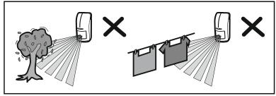
Don't install the detector closer than 3 meters from the moving objects (eg. tree branches, bushes, laundry etc.).
