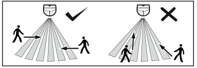
Install the detector so that the expected movement of an intruder will be across the coverage pattern.
