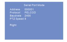
Note: In serial port mode, many PTZ operations can be done, such as change direction, zoom in/out, adjust IRIS, call or set preset, etc.
