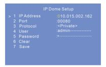
♦ IP address: Enter the IP address of the PTZ camera. This IP address must be in the same local network segment with the local IP address of the network keyboard.
