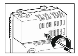
2. Remove the cover of power supply terminals.
