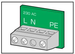
11. Screw the wire fastening element.
