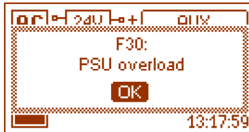
Fig. 13. Information that power supply is overloaded.
